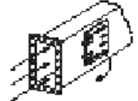
Bolted Access Door in Duct
