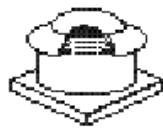
Screen on Roof Ventilator
