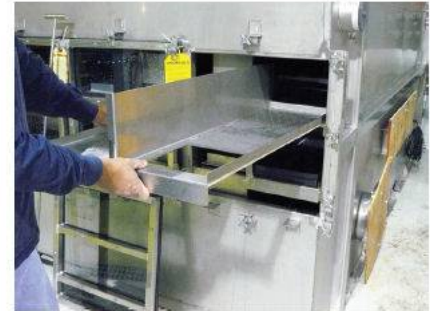
3. Remove downcomer and then fully remove the front tray and set aside.
