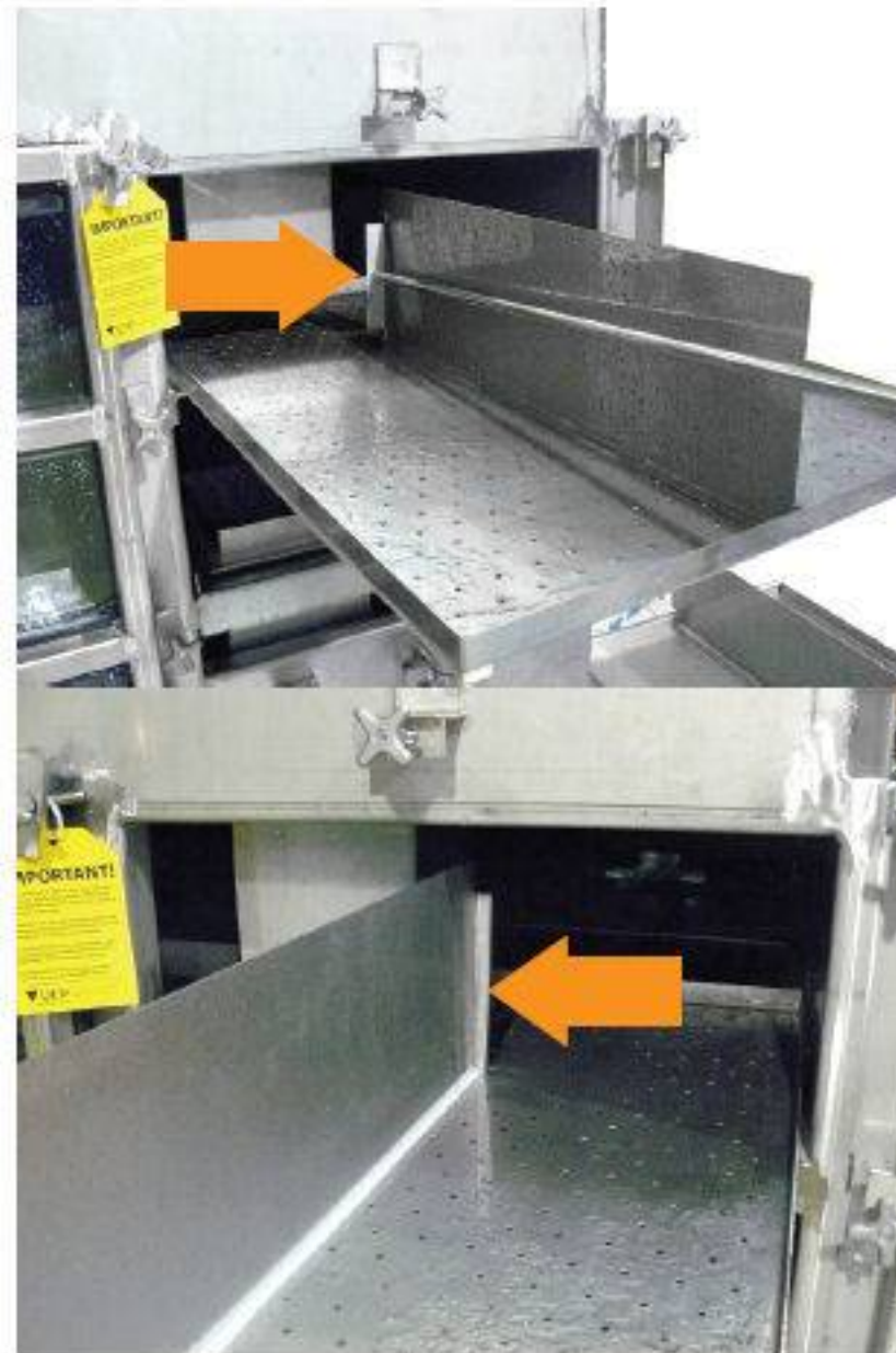
5. Extend the Tray Remover Tool inside the Air Stripper housing and "hook" the channel end around the back of the divider (vertical upright part on each tray).
