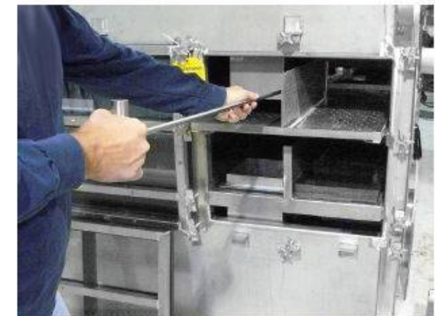
6. Firmly pull on Tray Remover handle and pull rear tray out towards front of Air Stripper access door / hatch opening.
