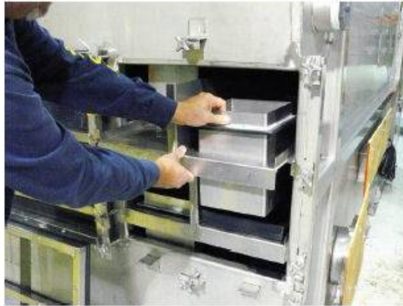
2. Pull out the front tray while slightly lifting up on the downcomer (of the tray being removed) in order for the downcomer to clear the seal pot pan area of the tray below.
