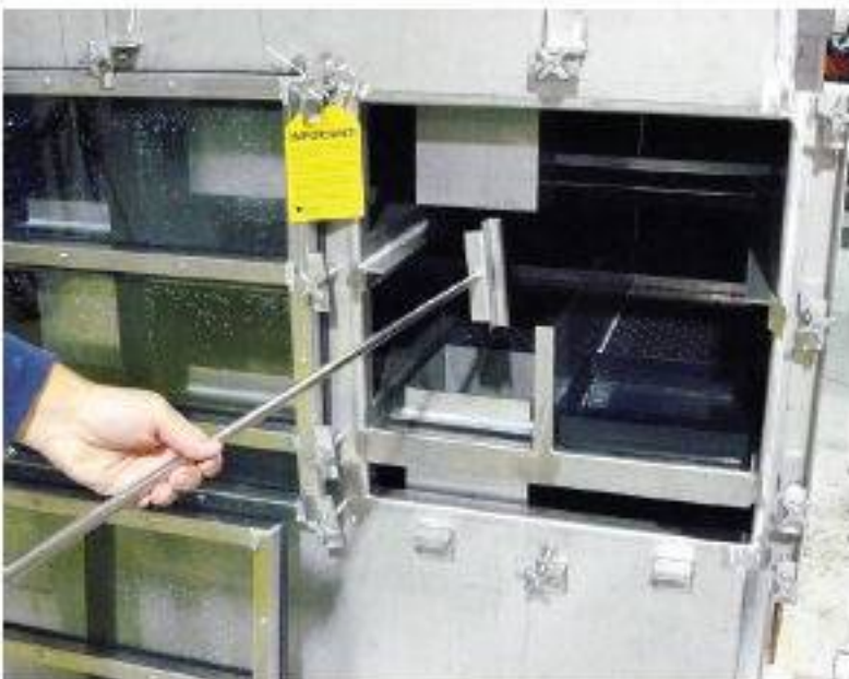
4. Grab Tray Remover Tool "T" Handle in your hand and position the "channel" or hook end in a vertical position.
