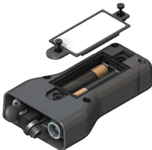
Figure 18 - Affinity Battery Access
